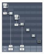
Please note that the **Input** is also present on the **FM Matrix**. You can use it as modulator and carrier as if it where a normal Operator. This opens a lot of new possibilities for using the FM8 as an effects processor.
