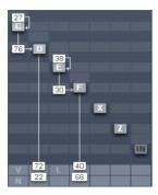
The **FM Matrix** can be found in almost all Expert windows. It is the heart of the FM8 synthesis engine where the modulation relationships between Operators are defined. You can arbitrarily take any Operator's output to modulate the frequency of any other Operator using a concise interface.
