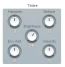
**Harmonic** changes the harmonic content (by adjusting the Operator Ratios). Depending on the patch, the changed harmonics may be somewhat atonal.
