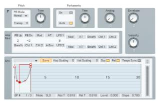
All aspects of pitch are assembled on the **Pitch** window. Dial in the main pitch, Portamento and the Pitch Envelope.
