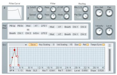
This special-case Operator is a signal processor that contains two separate filters (each a 2-pole 24dB/oct multimode filter), which can be combined in almost any imaginable configuration. Yes, FM synthesis finally has a great-sounding, analogue-style multimode filter.
