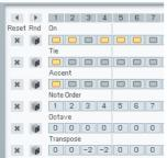
The **Pattern Editor** is the place where you actually develop your sequences. It consists of a grid with the columns representing the individual steps and each row controlling one of the six parameters. The steps and the binary parameters can be activated / deactivated by single mouse-clicks. The parameters offering more than one state present a menu with the possible values.
