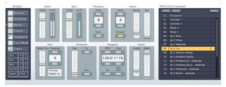
The **Master** Window provides access to the global parameters of the FM8. Here you find things like the main levels, Polyphony settings, global pitch controls and the MIDI controller assignments.
