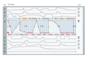
An important aspect of a vivid FM Sound is the Envelopes controlling the amplitude of modulators and carriers. The **Envelope** window gives an overview over all envelopes and still maintains the possibility to edit them. You can also display a single envelope filling out the complete window or even stack multiple envelopes in one single graph.
