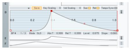
In the next step **deactivate the link buttons** and switch to the **Envelope** of **Operator D**. Grab the **Slope handle** of the **Attack** phase (the red dot) and dial in an **exponential slope**. Play some keys and you will hear that the **harmonics** are being **faded** into the Sound along the Envelope of Operator D, which is a modulator. This makes the Envelope of Operator D similar to a filter Envelope.
