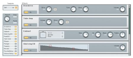
The FM8 provides a complete set of high-quality effects to be used in your sound designs. The Effects units are displayed in a **rack** of virtual devices and the **signal flows** serially from top to bottom.
