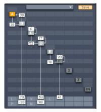
Operator A modulates Operator B, which is a modulator for Operator C. Operators C, D, and E all modulate Operator F, which serves as a carrier, and feeds the output. Note that Operator D has feedback.
